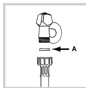
1. Insert seal A into the end of the inlet hose and screw the latter onto a cold water tap with a 3/4 gas threaded opening (see figure). Before performing the connection, allow the water to run freely until it is perfectly clear.
