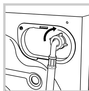
2. Connect the inlet hose to the machine by screwing it onto the cold water inlet of the appliance, which is situated on the top right-hand side of the rear part of the appliance (see figure).
