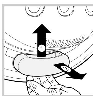
1. Remove the compartment by applying a light pressure to the lower part.
