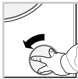
1. remove the protective casing on the lower part of the washing machine, turning it in an **anticlockwise direction** (see figure);
