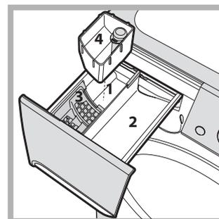
This function is particularly useful for the removal of stubborn stains. Insert extra compartment 4 (supplied with the appliance) into compartment 1. When pouring in the bleach, be careful not to exceed the "max" level marked on the central pivot (see figure). To bleach laundry with no other washing action, pour the
