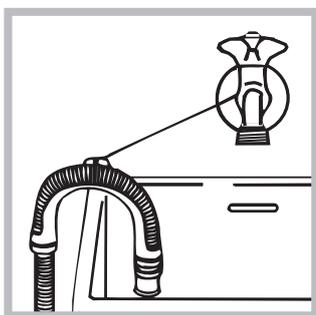
alternatively, rest it on the side of a washbasin or bathtub, fastening the duct supplied to the tap (see figure). The free end of the hose should not be underwater.
