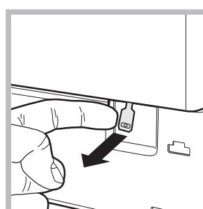
4. pull outwards using the tab as indicated in the figure, until the plastic tie-rod is freed from its stop
