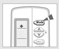
2 If the is not displayed at the top of the remote control, press the Mode button on the remote control one or more times until it appears.
