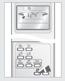
The air conditioner can generate anions with an ionizer in the indoor unit. Since it is an additional function, you can select it any mode, even when the air conditioner is turned off.
