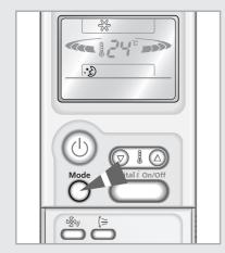
The Sleep Timer can be used when you are cooling or heating your room to switch the air conditioner off automatically after a period of six hours.
